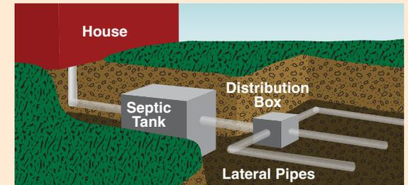
*Septic tanks are designed to allow bacteria and enzymes to biodegrade organic waste. This amazing process actually converts waste into water, carbon dioxide and small amounts of mineral matter!*
