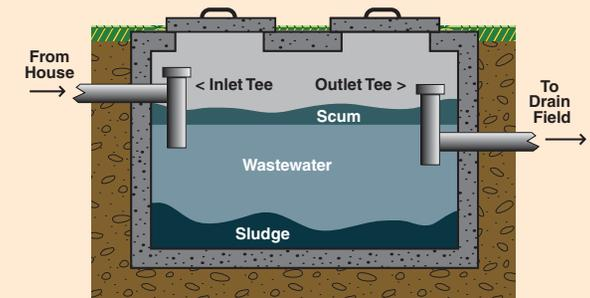
*Incoming solid matter sinks. Soap and grease float. The tank has an outlet baffle to hold in undigested waste. Only clean water should leave the tank and enter the lateral pipes.*
